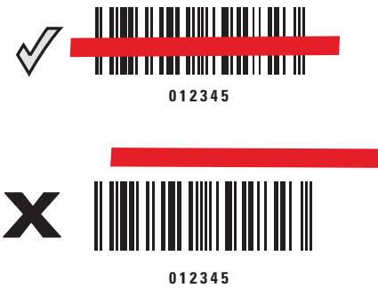
Figure 3-3 Scanning Orientation with Aiming Line
